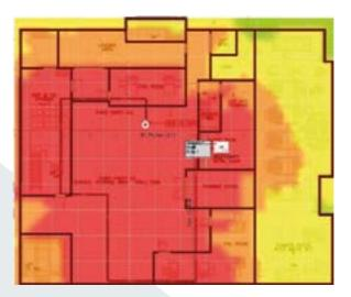
Prior to any physical installation on the platform, we use a sophisticated program to ensure that the final design of the DAS will provide the necessary and expected radio coverage. The program will visualize the distribution of radio signal throughout individual decks and compartments on the platform. If any areas are found to be poorly covered by the DAS, the cables or antennas can be repositioned to solve the problem.
