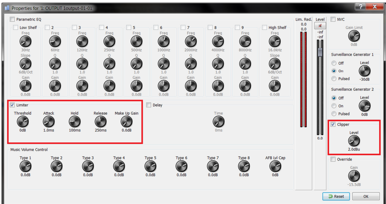
Figure 8 VIPEDIA-12 Dynamic Configuration Tool – Output Limiter and Clipper
