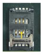
Figure 1: Retention Clip Closed
