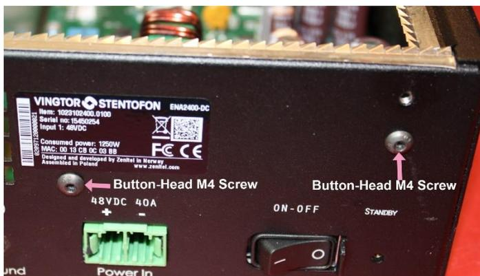
Remove the PSU according to the following procedure:
