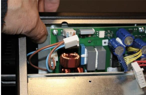
3. Push the lower edge in and align the screw holes on the PSU with the corresponding mounting holes on the cabinet floor.
