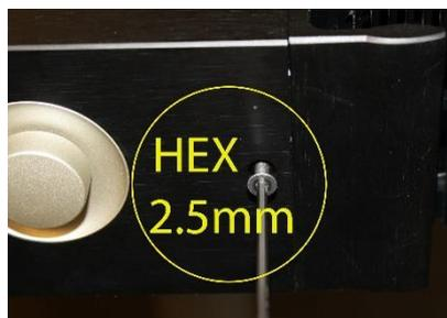
3. Using extractors to hold the screws, pull the front cover out and tilt it down forcefully to access the inside of the unit.
