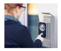
An example of integrating access to control and video management systems is the install of an intercom at the door. Entry requires communication between a visitor and an operator. This solution allows the receptionist or an employee to verify and remotely operate the door for a visitor.
