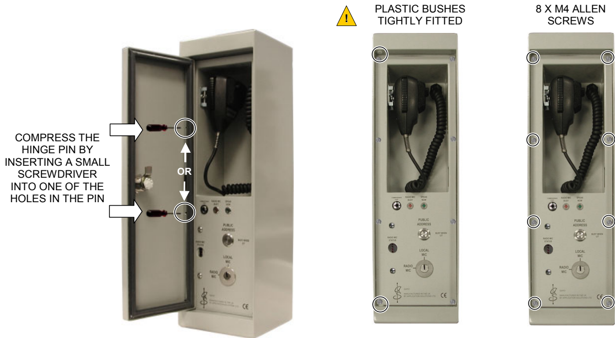
Figure 28 SAP01 Door and Front Panel Fixing
