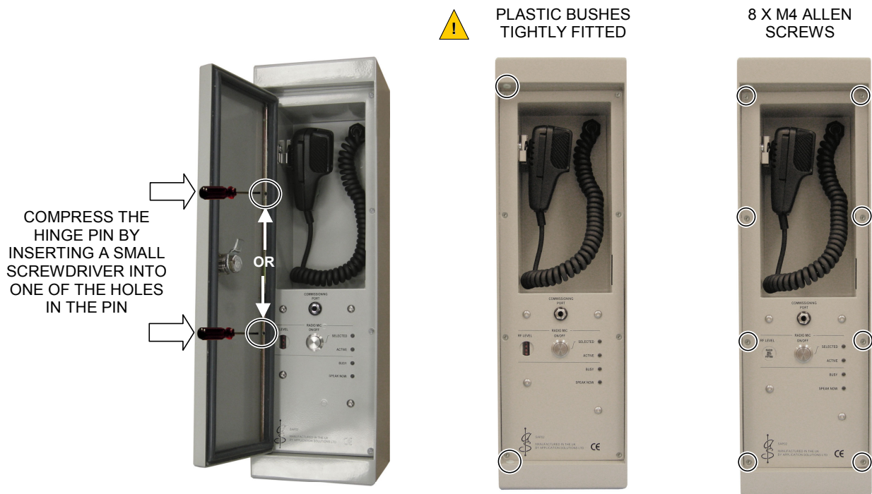
Figure 5 SAP02 Door and Front Panel Fixing
