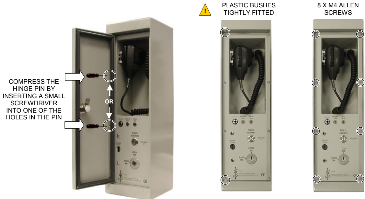
Figure 11 SAP01 Door and Front Panel Fixing
