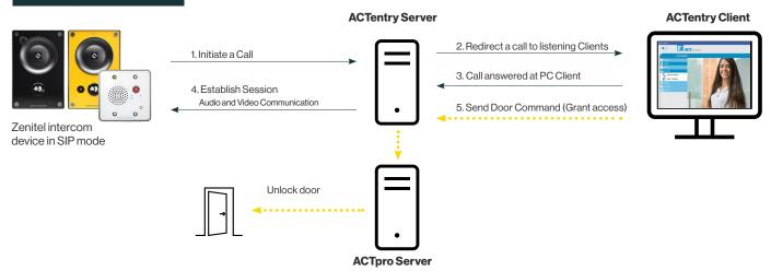
The Zenitel intercom devices are connected to an ACTentry server, which enables the association with access control doors and the communication to and from the operators using the ACTentry client. To perform door actions and grant access, ACTentry communicates with the ACTpro access control software, enabling operators to:
