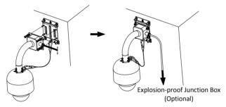
Figure 2-9 Secure the Bracket
