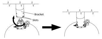
Figure 2-6 Rotate the Bracket
