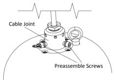
Figure 2-11 Insert the Screws
