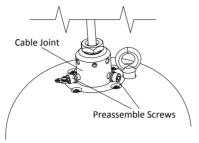
Figure 2-5 Insert the Screws
