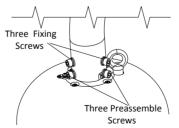
Figure 2-7 Secure the Speed Dome
