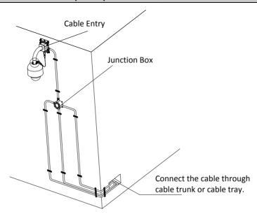
Figure 2-2 Cable Wiring Diagram
