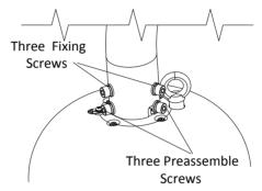
Figure 2-13 Secure the Speed Dome
