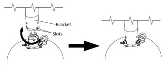
Figure 2-12 Rotate the Bracket
