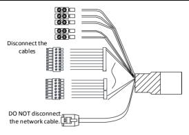
Figure 2-3 Disconnecting the cables
