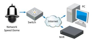
Figure 3-2 Wiring over LAN
