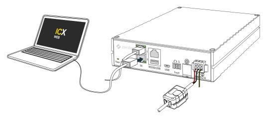
**Connect to web server - ICX Web.** The ICX-510-IA comes with an embedded web server which provides functions for system configuration, monitoring and upgrade.
