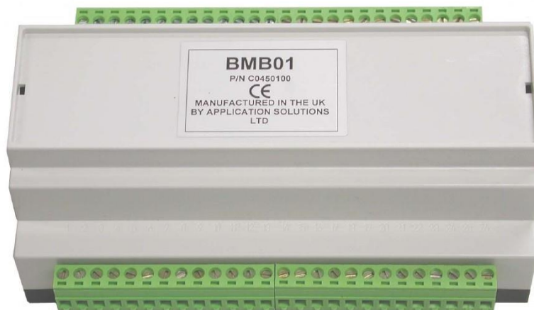
Figure 3: BMB01 GPIO Unit
