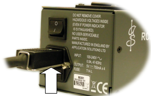
RETAINING CLIP SECURING THE CABLE
