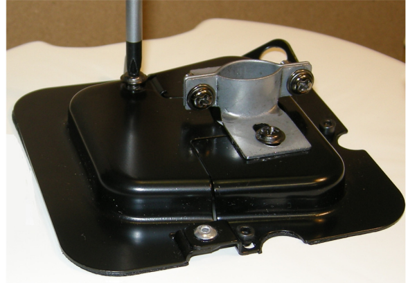
Top view of loudspeaker – undoing top plate screw
