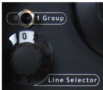
Figure 3: Group and Line Selector
