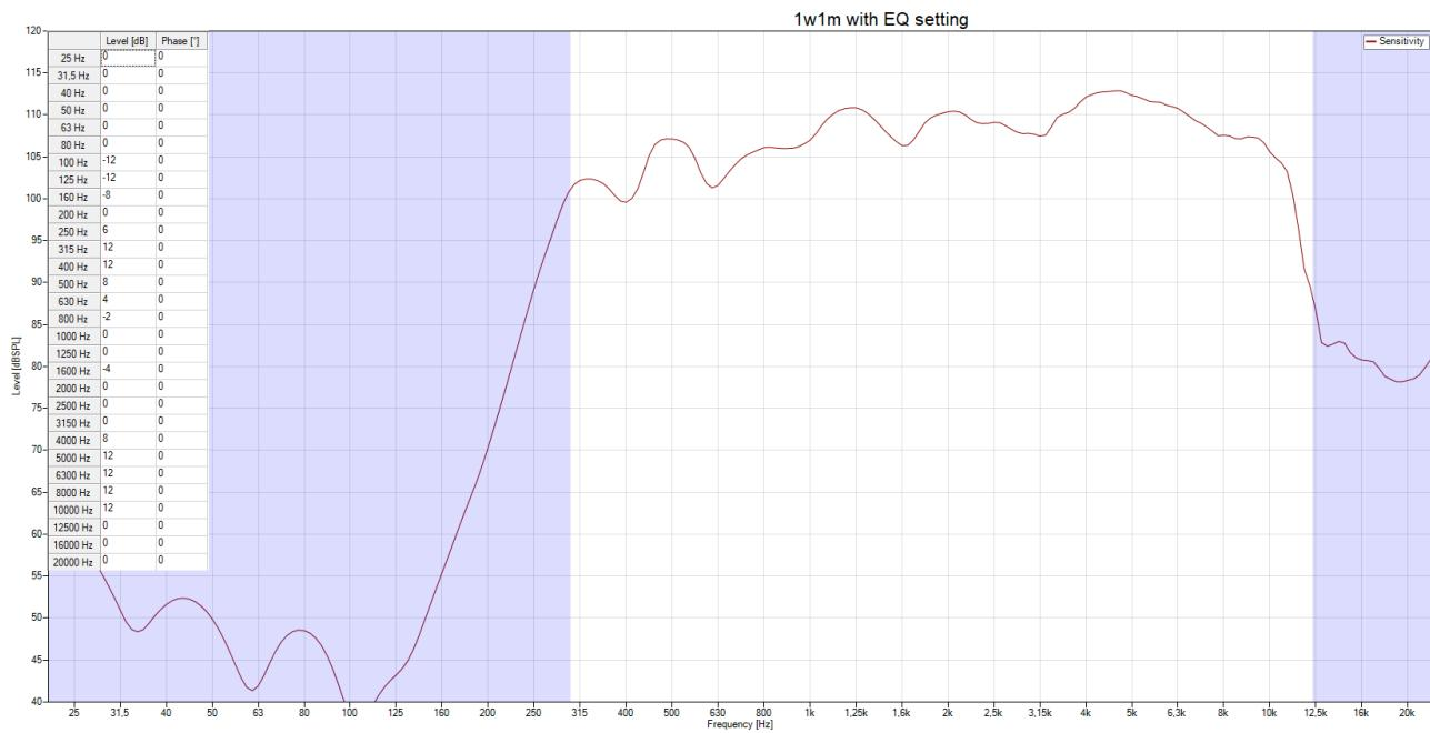
**FREQUENCY RESPONSE DIAGRAM—MAXIMUM SPL (Vrms 1 min, 1m)**
