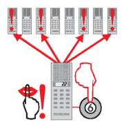
Master stations programmed for Silent Alarm can make an emergency alarm call to a predetermined group of stations. The call can also be initiated by a concealed button or a foot-switch. Any station can be programmed to receive Silent Alarm calls.
