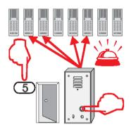
Programmable in 1-button substations where the call button activates the Doorbell function.
