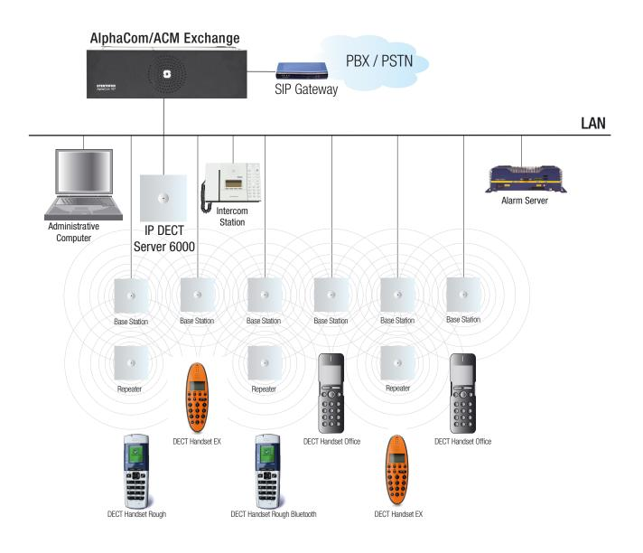
Figure 1 IP DECT 6000 System Configuration
