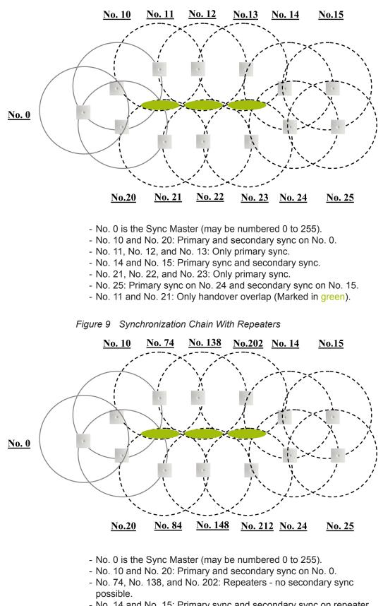
Figure 8 Sync Chain With and Without Secondary Sync Ways
