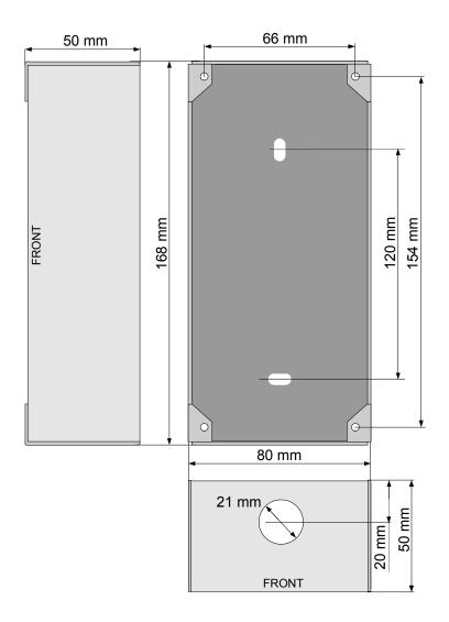
Figure 5 IP Substation - Flush Mount Backbox
