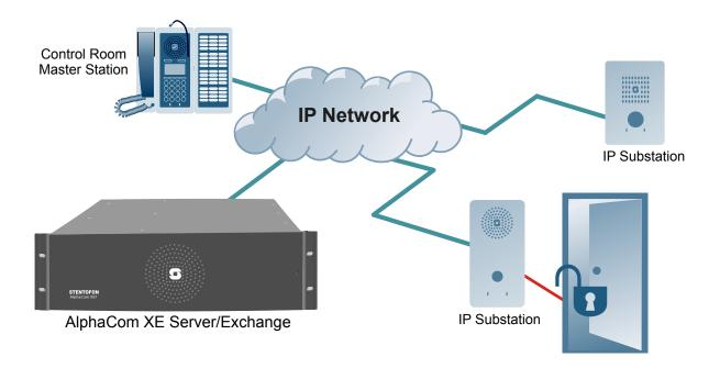
Figure 1 STENTOFON Security and Communication System
