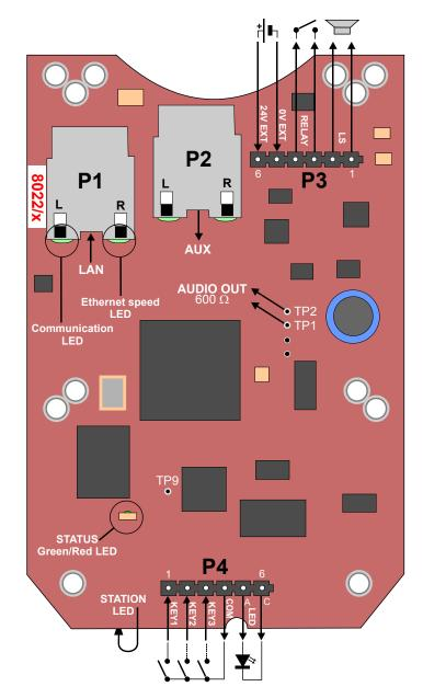
Figure 3 Substation Board Connections
