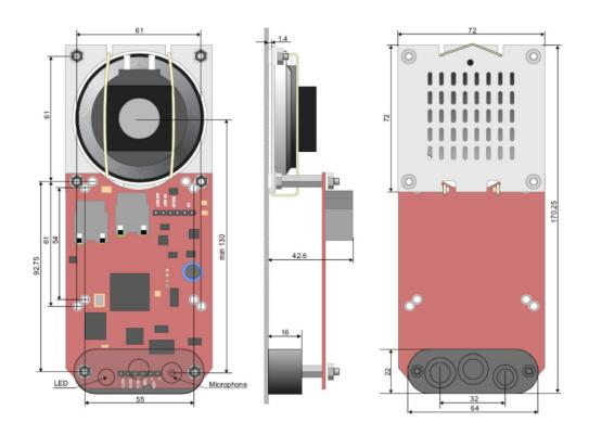
Figure 9 IP Substation Kit Mounting Dimensions (mm)
