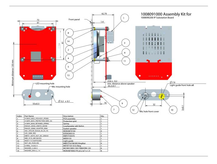
Figure 11 IP Substation Assembly Kit Mounting Dimensions
