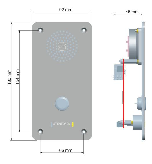
Figure 4 IP Substation Dimensions
