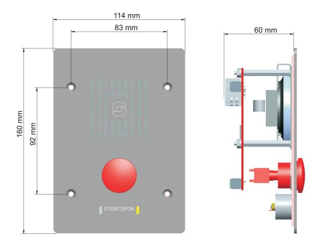
Figure 7 IP Substation (3 Gang) Dimensions
