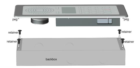
The station is securely fastened to the backbox using the four retention pegs supplied.
