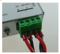
For the first converter unit on the configuration, one connection can be used to connect the power supply, while the other can be used to connect to the actual star configuration. The power supply may be connected at any point on the star configuration, i.e. it can be connected to any of the Flowire Converters on the star configuration.
