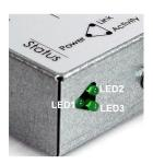
**LED1 - Power**: This LED is lit when the converter is receiving enough power for powering up.
