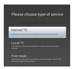
There are 3 modes one can choose from: **Internet TV**, **Local TV** and **Free mode**. In the **Internet TV** mode, the set-top box is connected to the provider's IPTV middleware server over the internet. In the **Local TV** mode, the set-top box is connected to an IPTV middleware server available in the provider's local network. In the **Free mode** there's no connection to an IPTV middleware server.
