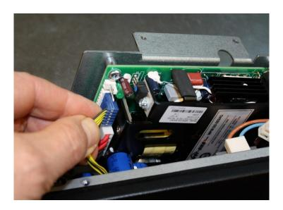
6. Lift and turn the AC-DC PSU, freeing it from the cabinet cavity
