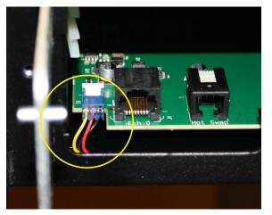
2. Push the plug into the cavity on the left side.
