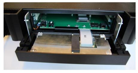
4. Remove the top cover by unscrewing the 8 Torx screws using a T10 bit.
