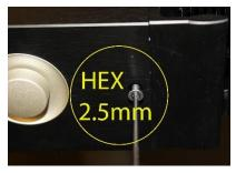
3. Using extractors to hold the screws, pull the front cover out and tilt it down forcefully to access the inside of the unit.
