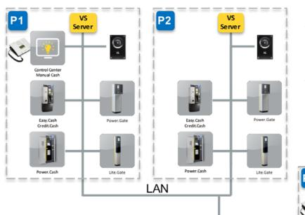
**MULTI SITES:** Intercom system with multiple intercom servers installed on different networks – deployed on one large facility or many remotely located parking facilities.
