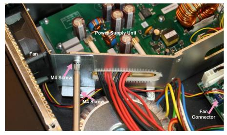
2. Use a PZ2 bit to unscrew the side M4 screw and bottom M4 screw on the flange of the fan
