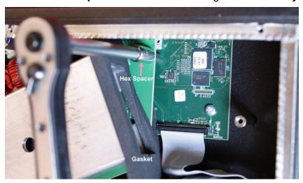
Figure 3: Removing Hex Spacer
