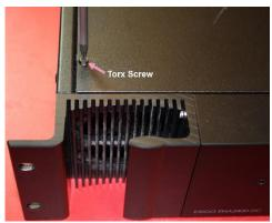
Figure 1: Removing Top Panel
