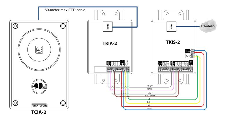
• Using the 8-wire cable, connect the pins on the TKIA-2 to the corresponding pins on the TKIS-2 according to the schematic above.
