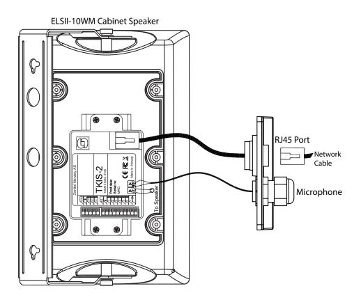
The ELSII-10WM comes with an external RJ45 port that is pre-wired to the TKIS-2 kit inside the unit.
