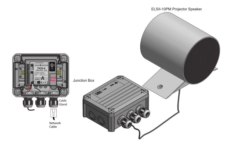
The ELSII-10PM comes with an external junction box that houses the TKIS-2 kit and microphone.
