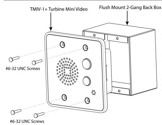
To attain the rated ingress protection of IP44, flush mounting of TMIV-1+ must only be done on a surface that is completely planar, smooth, and clean. Any surface irregularities must not exceed 0.5 mm. If this is not achievable in a reliable manner, appropriate sealant or filler should be applied to seal the gap between the station and the wall. Optionally, the on-wall back box TA-32 could be used.
