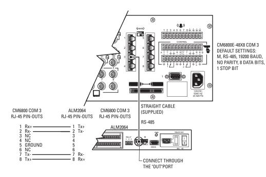
Figure 19. Connecting a Single ALM2064 Alarm Interface Unit
