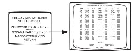
Figure 50. Scratchpad Sequence Screen
