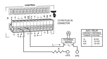
Io = OPERATING CURRENT OF THE EXTERNAL DEVICE (MUST NOT EXCEED AUX 1 CURRENT RATING.)
