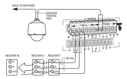
Figure 9. PTZ Control Connections
