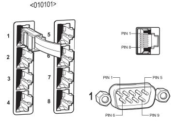
Figure 12. Communication Port Inputs
