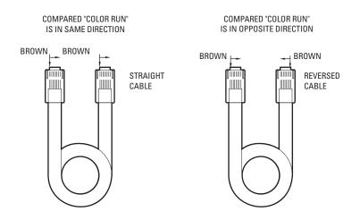
Figure 17. RJ-45 Cable Types
