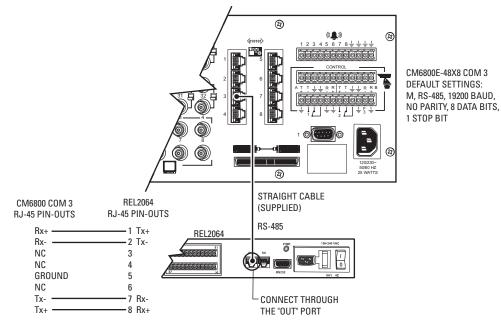
Figure 20. Connecting a Single REL2064 Relay Interface Unit
