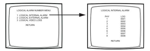
Figure 57. Assign Satellite Logical Alarm Numbers
