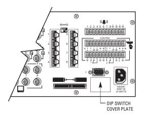
Figure 65. DIP Switch Cover Plate
