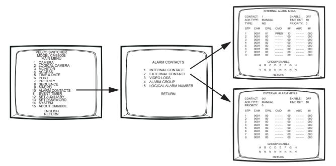
Figure 35. Program Internal and External Alarms
