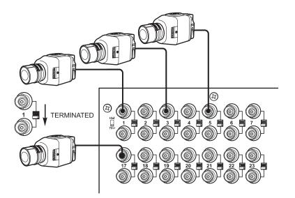
Figure 7. Connecting Terminated Video Sources
