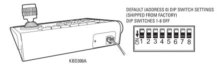
Figure 14. Data Cable Plugged into Local Keyboard
