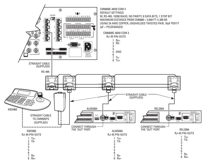
Figure 22. Connecting Multiple M Devices – Remote Connection
