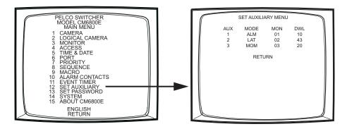
Figure 38. Program Auxiliary Outputs
