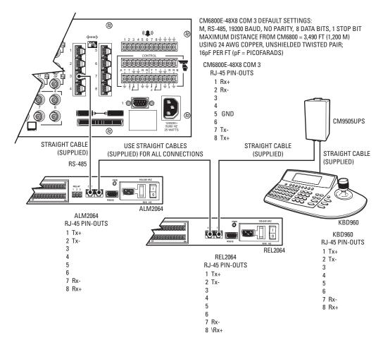
Figure 21. Connecting Multiple M Devices - Local Connection
