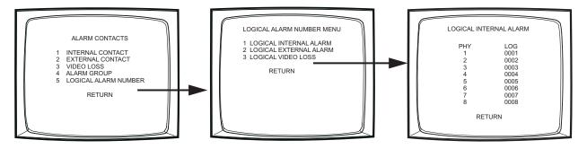
Figure 37. Assign a Logical Alarm Number
