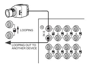
Figure 8. Connecting Looping Video Sources
