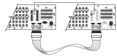
Figure 28. Data and Video Connections Between CM6800E-48X8 Units
