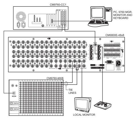
Figure 53. Data and Tie Line Connections Between CM6800E-48X8 and CM9700/CM9740/CM9760
