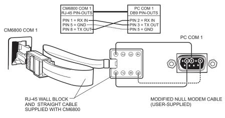
Figure 24. PC Connection to RJ-45 Port
