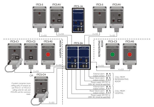
Calling system type ITCS-A is realised using control unit type ITCS-IA (single) or ITCS-2A (double), arbitrarily number of calling units type ITCS-C1, ITCS-C2, ITCS-C3 and/or ITCS-C4 and reset unit type ITCS-RS. If calling unit type ITCS-C4 is used, it comprises also the call reset function, so there is no need for further reset units. System can be additionally equipped with signaling units type ITCS-S and repeater units type ITCS-RI.
