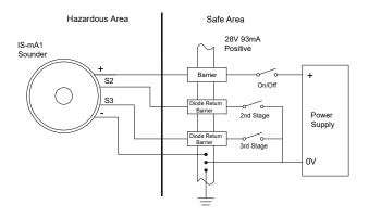
Fig 6 Multi stage alarm using Zener barriers.
