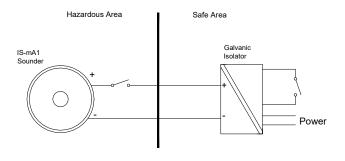
Fig 7 Single stage alarm using galvanic isolator.
