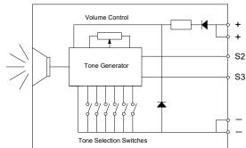
Fig 1 Simplified block diagram
