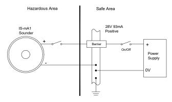
Fig 4 Single stage alarm using single channel barrier.
