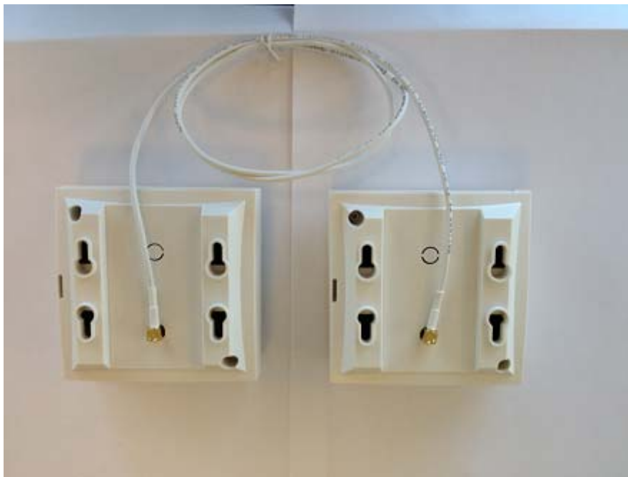
Figure 11 Connect Power to the Bottom of the Repeater and External Antenna Cable to the Rear of the Repeater
