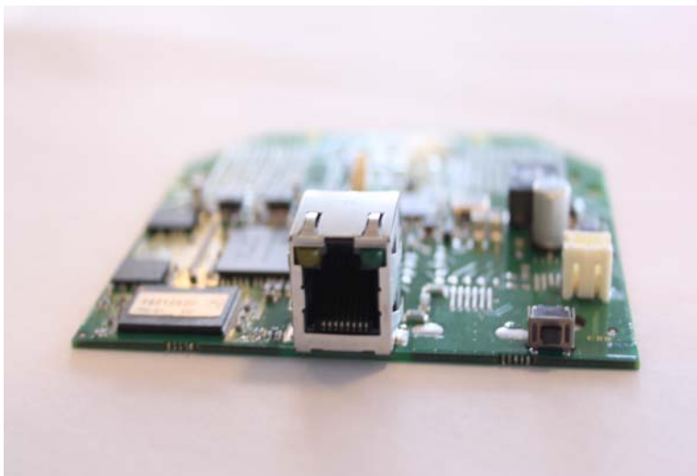
Figure 2 Add-on media resource for empty slot in a Server 6500 Rack
