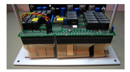
c. Gently pull the flexiprint connector(s) (The CIS 3102/3130/3131/3132 contains 2, the CIS 3100/3101 contains 1) downwards to disconnect the front module connection tail. Make sure the connector(s) come off evenly
