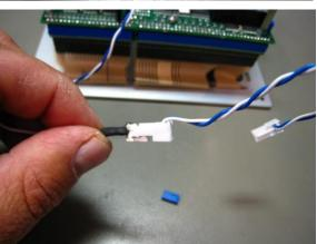
j. Tighten up the dimmer module cable and fasten the cable gland. Replace the backbox by sliding it gently towards the front. 2 cm from the end special care must be taken to not damage the flexiprint cable from the front module. The 97301-022 Dimmer board insertion causes this cable to bulge somewhat outwards. Use an finger or an edgeless device to force the flexiprint inside the box while pressing it in place.
