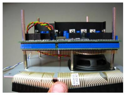
f. Next stage is to insert the flexiprint connector(s) into the pin header on the 97301-022
