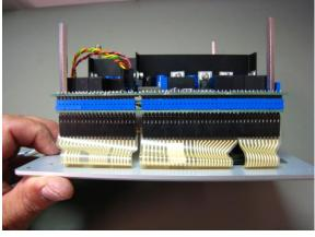
g. Pull the white/blue adjustment input wires up to the upper side of the main unit board beside the loudspeaker/vol.pots wires and secure to the spacer/support pillar as shown below
