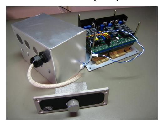
i. Remove the Blue jumper on the 97301-022 Dimmer board adjustment wires and connect the 9026 Dimmer module. The two connectors are equal and either of them
