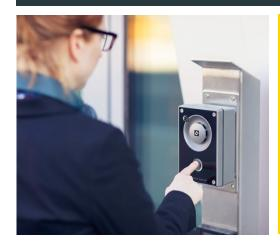
This feature automatically adjusts the speaker's voice, maintaining a constant volume level to the receiver, regardless of the speaker's distance from the station.
