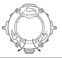
② Engage the attachment mounting screw of the camera with the camera mounting hole of the camera attachment and rotate the camera in the direction of the arrow to the "LOCK" position to secure the camera to the camera attachment without any backlash.
