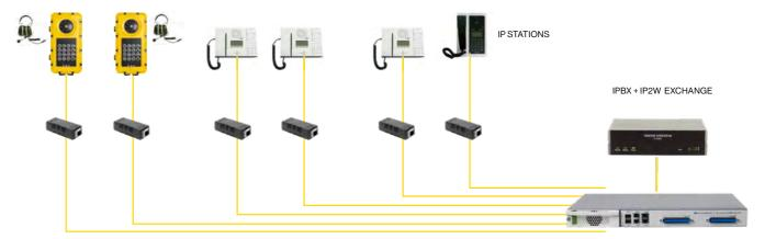
IP over original cabling, minimum 1 single pair cable required
